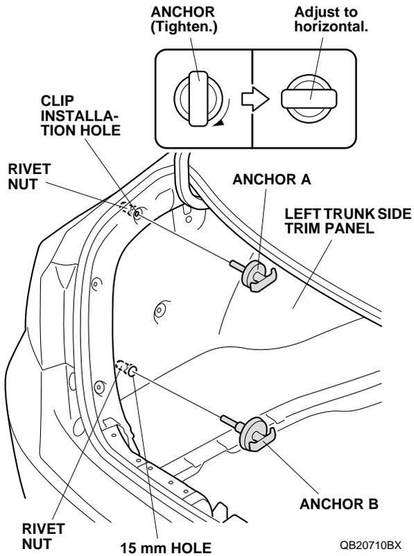
21. Using the right template, repeat steps 13 through 20 to install anchors on the right side of the vehicle.
