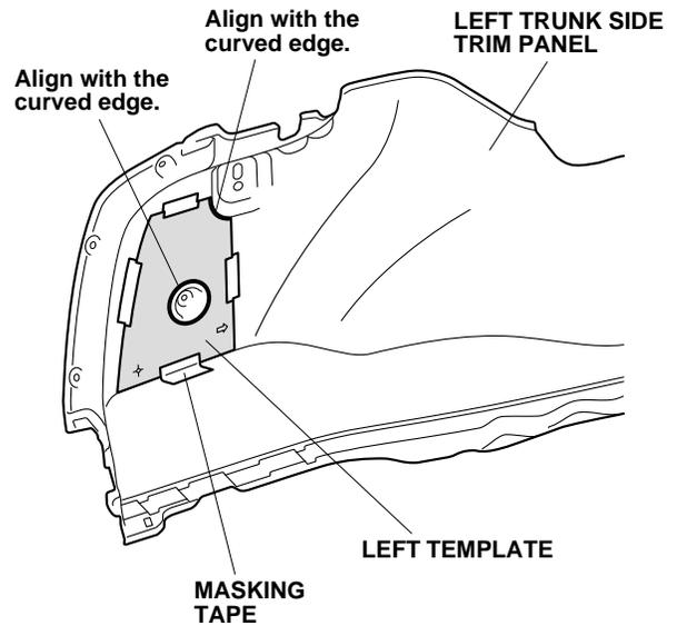
15. Using a felt-tip pen, mark the left trunk side trim panel through the hole in the left template. Remove the left template.
